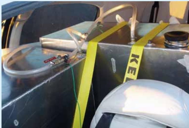
*Auxiliary fuel tanks inside the aircraft.*
